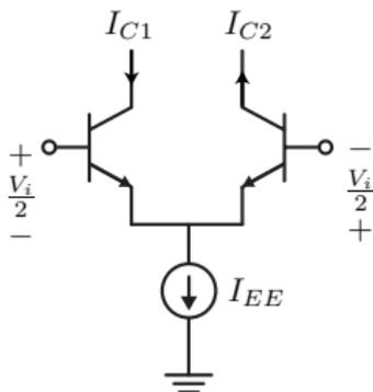
The differential pair is an important analog and RF building block.
