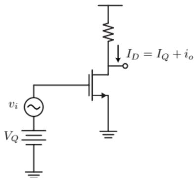
$$I_D = \frac{1}{2} \mu C_{ox} \frac{W}{L} (V_{GS} - V_T)^2$$
