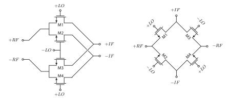
• Note that the Gilbert quad is really a folded ring. Thus the passive and active mixers are very similar. The main difference is how the quad devices are biased. In the Gilbert cell they are biased nominally in saturation and have DC current. In the passive mixers, they are biased near the threshold.
