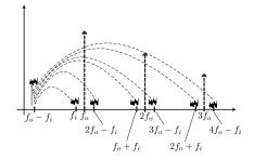
• PNoise is a noise analysis that takes the frequency translation effects into account. The simulation parameters are similar to PAC with the exception that we must identify the input and output ports (for noise figure) and the reference side-band, or the desired output frequency. For a mixer, this is k = -1.
