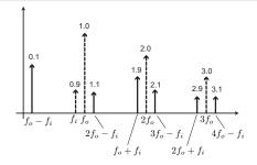
The input frequency f<sub>i</sub> is translated to frequencies f<sub>i</sub> + kf<sub>o</sub>, where f<sub>o</sub> is the beat (LO) frequency. The k = 0 sideband corresponds to the DC component of the LO signal (e.g. time invariant behavior). The non-zero components, though, correspond to mixing. E.g. k = -1 correspond to frequency down-conversion. k = +1 is the normal up-conversion. k = -2 is the 2nd harmonic mixing f<sub>i</sub> - 2f<sub>o</sub>.
