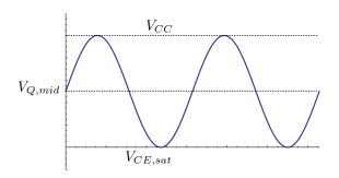
• We see that to avoid clipping, we should bias the transistor at the midpoint between  $V_{CC}$  and  $V_{CE,sat}$ . Thus
