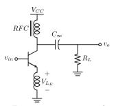
Emitter inductance has a detrimental effect on PA efficiency since it reduces the swing. The voltage across the emitter is given by
