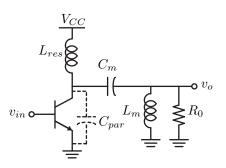
• In practice the collector inductor can double as a resonant element to tune out the collector parasitics. The coupling capacitor  $C_c$  can be replaced by a matching capacitor  $C_m$ .
