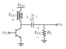
• Does this bother you? Recall that the voltage polarity across the inductor is given by dI/dt, which can go negative. Thus the collector voltage is equal to the supply minus or *plus* the absolute voltage across the inductor.
