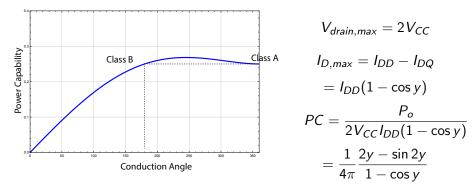
The power capacity of Class C is low at low conduction angles. Peak is Class AB.
