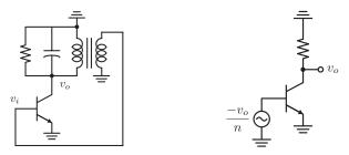
• At resonance, the AC equivalent circuit can be simplified. The transformer winding inductance *L* resonates with the total capacitance in the circuit. *R*<sub>T</sub> is the equivalent tank impedance at resonance.
