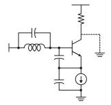
• Note that the collector can be connected to a resistor without changing the oscillator characteristics. In fact, the transistor provides a buffered output for "free".
