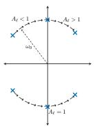
• We see that for  $A_{\ell} = 0$ , the poles are determined by the tank Q and lie in the LHP. As  $A_{\ell}$  is increased, the action of the positive feedback is to boost the gain of the amplifier and to decrease the bandwidth. Eventually, as  $A_{\ell} = 1$ , the loop gain becomes infinite in magnitude.
