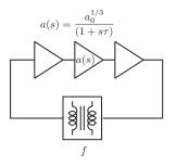
• As an example, consider a forward gain transfer function with three identical real negative poles with magnitude  $|\omega_p| = 1/\tau$  and a frequency independent feedback factor f
