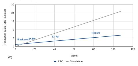
Developing an ASIC using a 65nm process cut power demands and cost for a disposable patient monitoring device - with Rol after 1 million units
