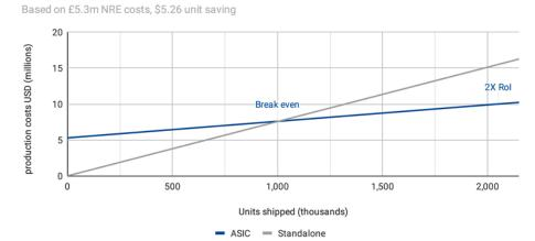
5. ASIC or off-the-shelf components – the economics behind the choice for a healthcare monitoring IoT system. Conversely, using off-the-shelf components would have meant both the high power and the high unit cost would have killed the product.
