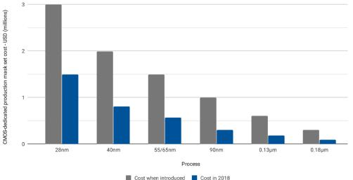
Using mature technologies cuts the mask set costs significantly: 2018 vs cost when each technology was introduced
