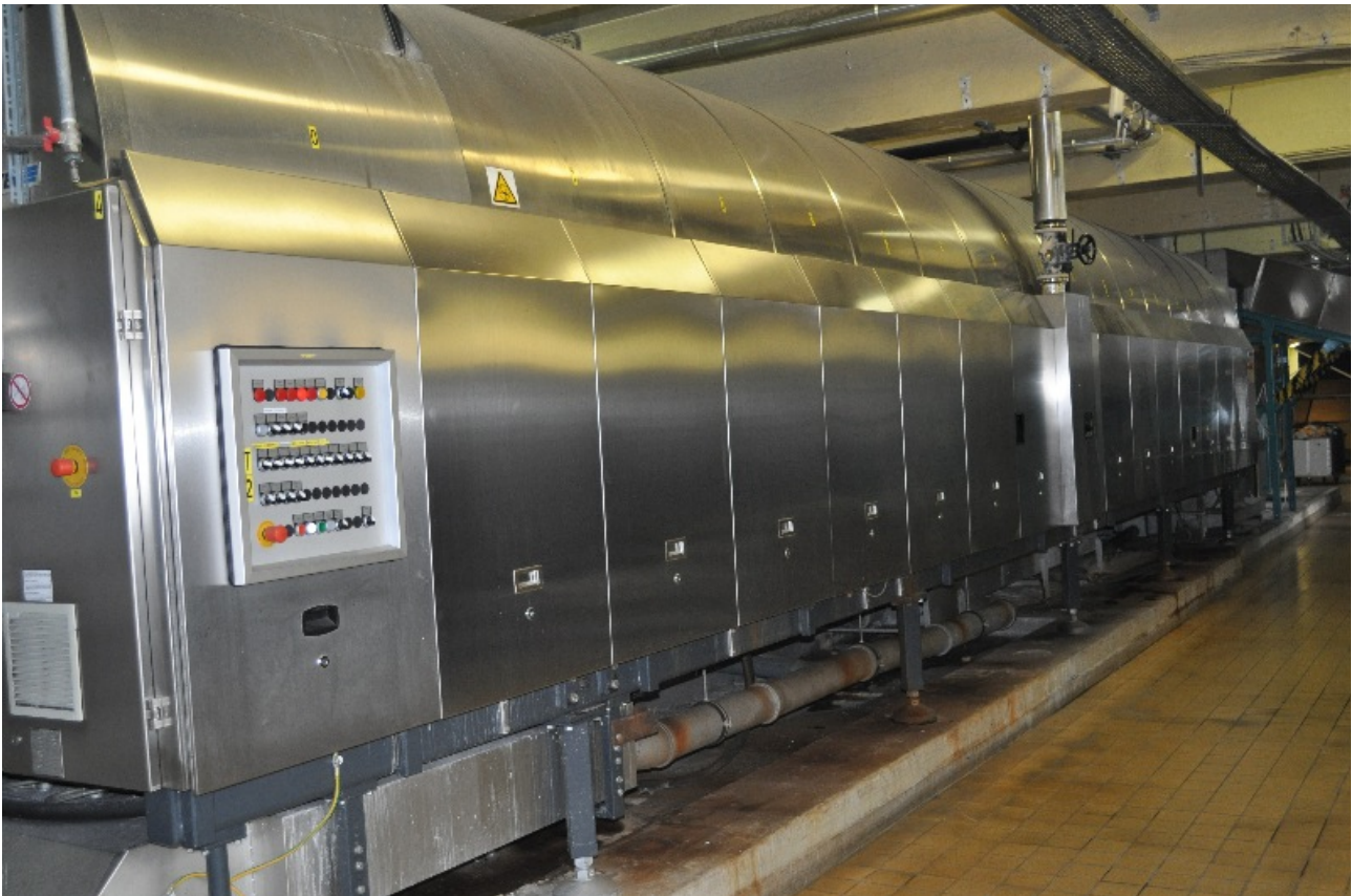
A typical CBW - this is a 50kg 14 compartment model, capable of washing up to 35 tonnes per day
