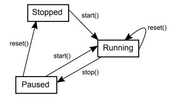
We have a model of the behavior of our chronometer with the different states it can reach according to the different actions we can perform. However, we have not modeled how these states are implemented in the program (is this a C enumeration? a particular program point in the source code?), nor how the computation of the elapsed time is done (a single variable? multiple ones?). It would then be difficult to specify properties about our program. We could add some information:
