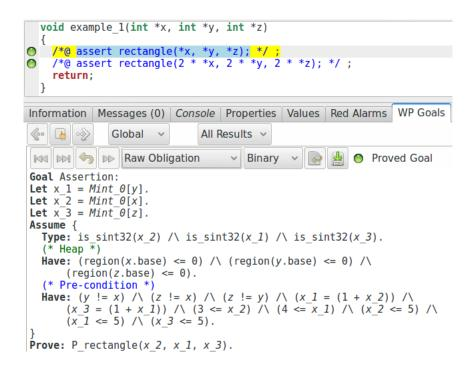
That is to say the different constraints we have stated as a precondition to the function (note that the values are not exactly the same, and some more properties have been specified). What is more interesting is having a look at the verification condition generated for the second
