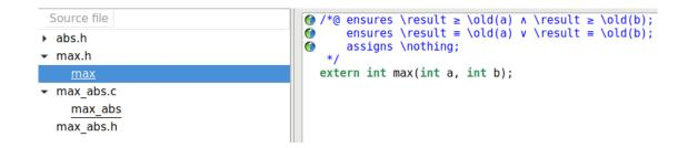
These bullets indicate that, since we do not have the implementation of the function, the postcondition of the function is assumed to be true. It is an important strength of the deductive proof of programs compared to some other formal methods: functions are verified in isolation from each other.
